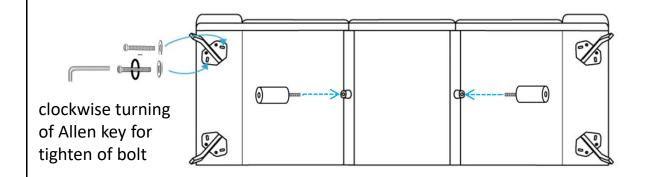
Step3: Remove protective packaging from the 3-Seater backrest packaged individually. Then tighten the backrest to the seat with bolts (f), washers (g) and spring washers (h) by Allen key (e).
