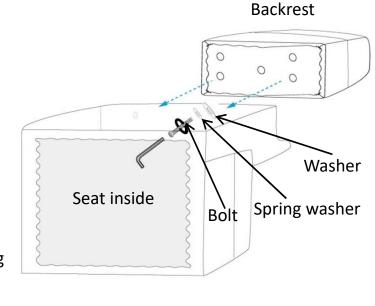
clockwise turning of Allen key for tighten of bolt
